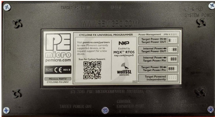
Figure 17-4: Rear Cyclone Case, Five Screws
