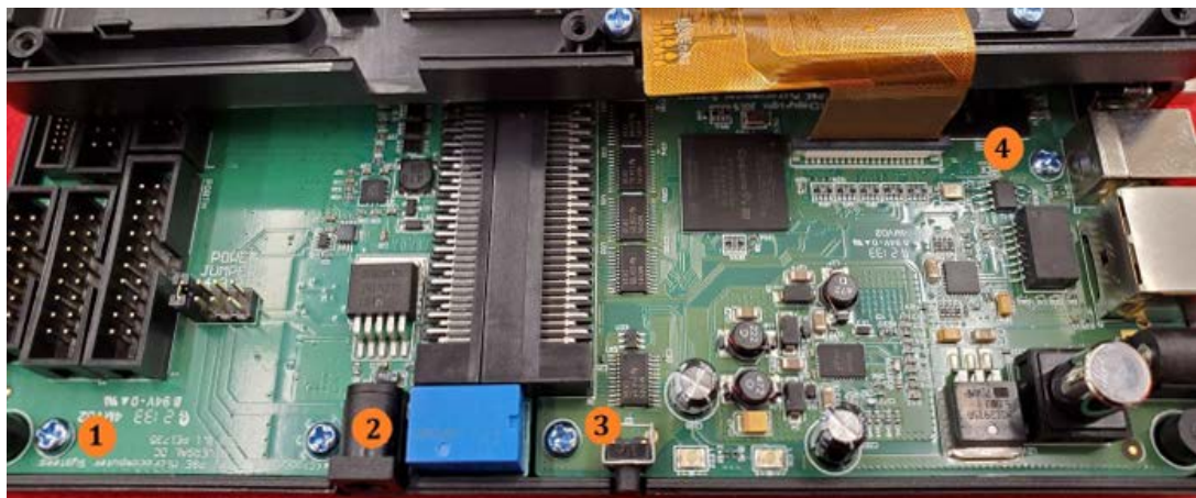
Figure 17-5: Bottom Half of PCB, Four Screws
