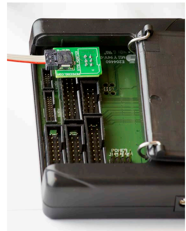
Figure 3-27: STM8 Adapter: 1) Bottom, 2) Top, 3) Connected To 6-Pin Header of Cyclone_Universal_FX (Adapter Sold Separately)
